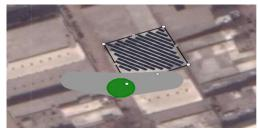
eventually, the panel gets damaged through heating. The efficiency of a panel at any time reduces in direct proportion to the area of the shadowed part of the panel. Sometimes even panels not in shadow zone get heated as they try to compensate for the power loss. Most often the damaged panels are not covered under warranty, adding to the operations cost of the plant.
